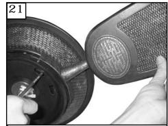
Check the motor for plastic shipping stabilizer tabs, and remove them if they are present. The screws, washers and motor pads are preinstalled to the blade holders. Attach blade assembly to motor and tighten screws securely.
